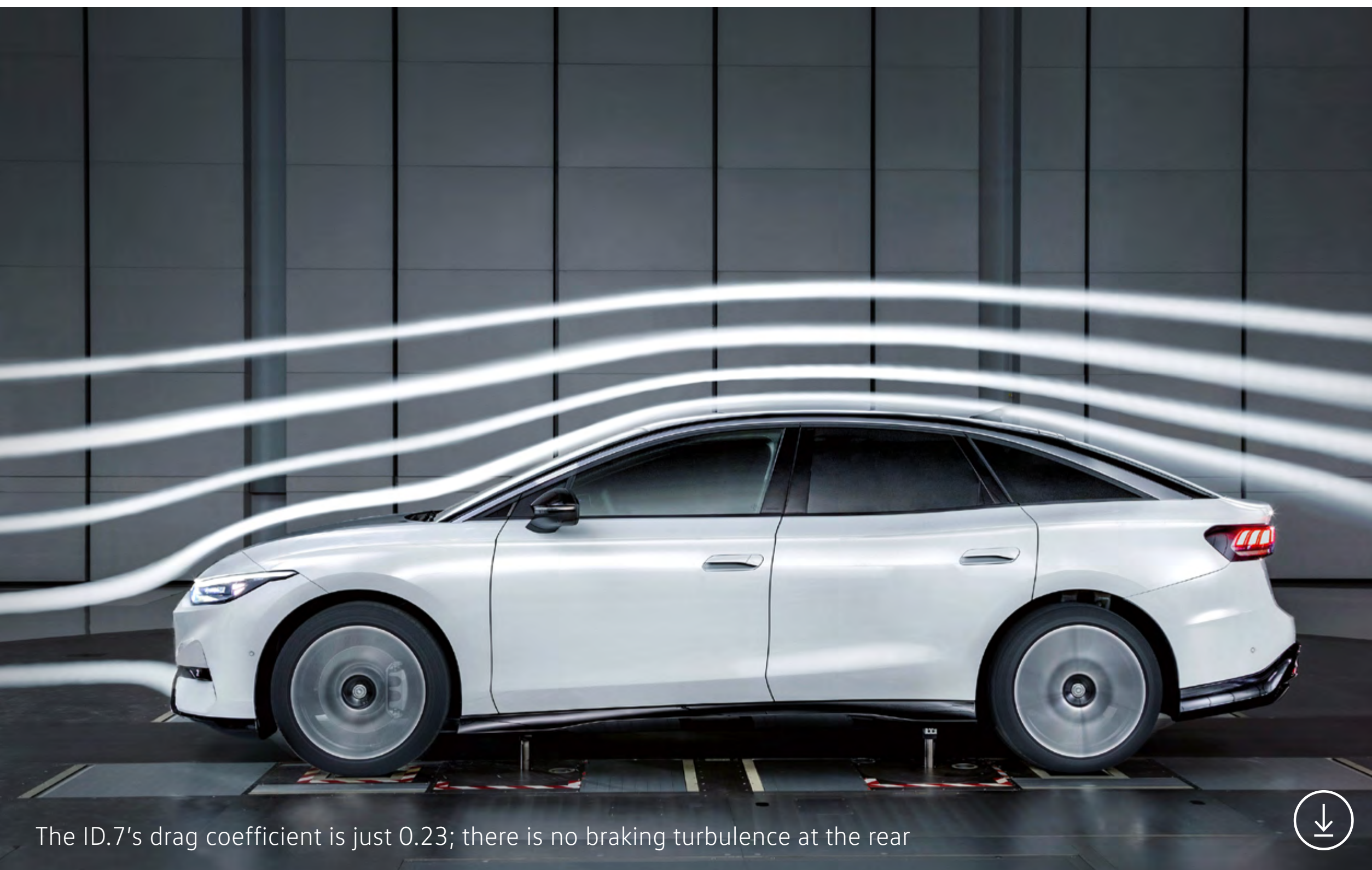
The aerodynamic interplay of drag coefficient and frontal area (2.45 m 2 ) increases the range
