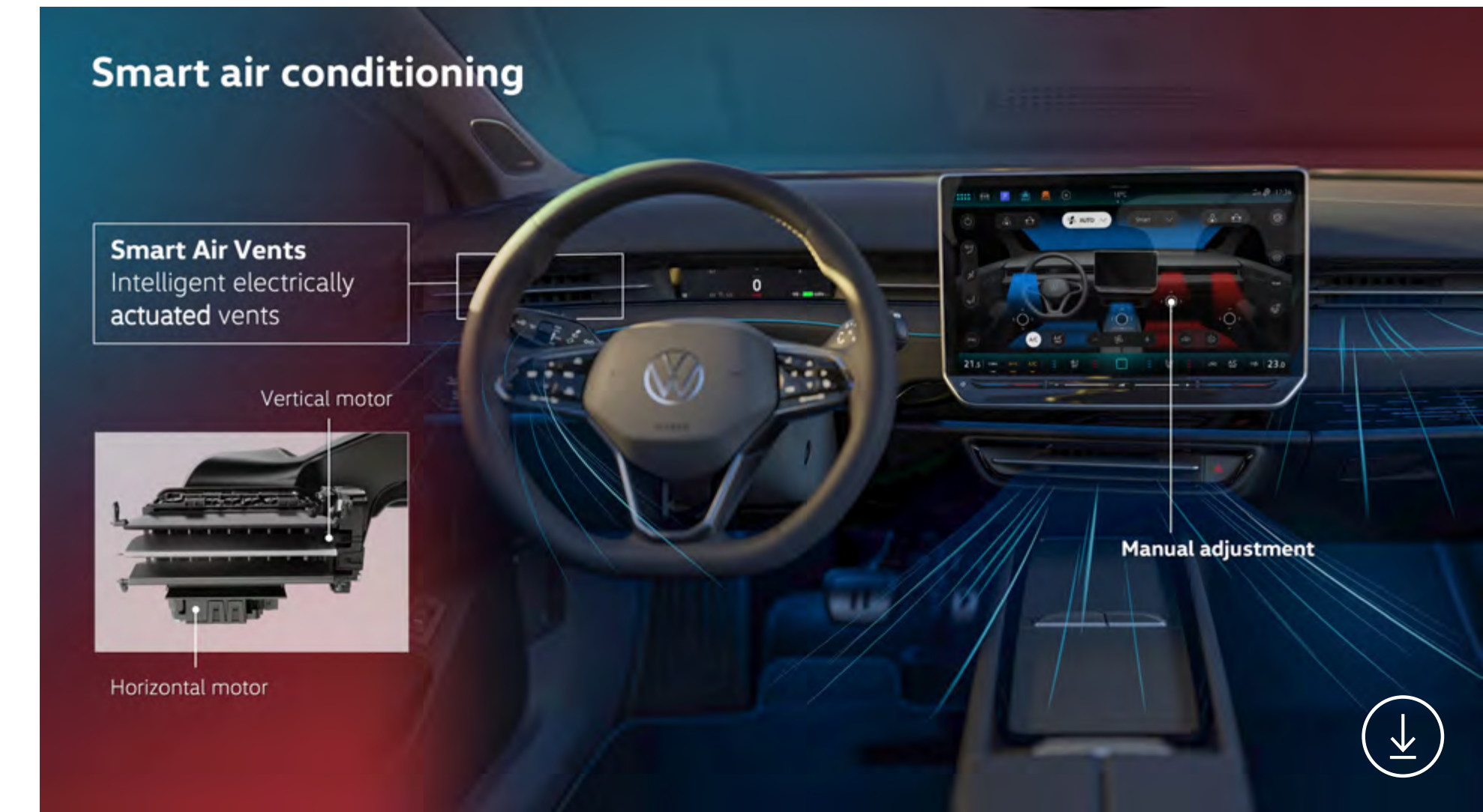
The air conditioning system can be controlled by voice and on the infotainment screen
