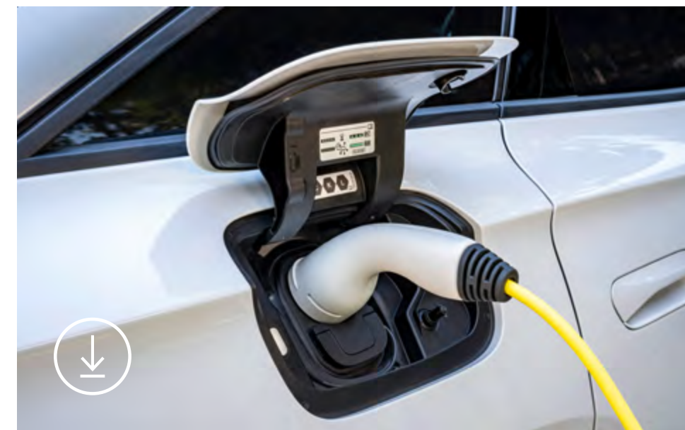
The charging socket flap opens upwards so the socket is always easily accessible.
