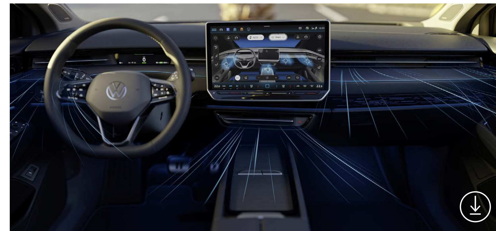
Controls for the intelligent air vents of the ID.7 Pro S 1 and ID.7 Tourer Pro S 2 .
