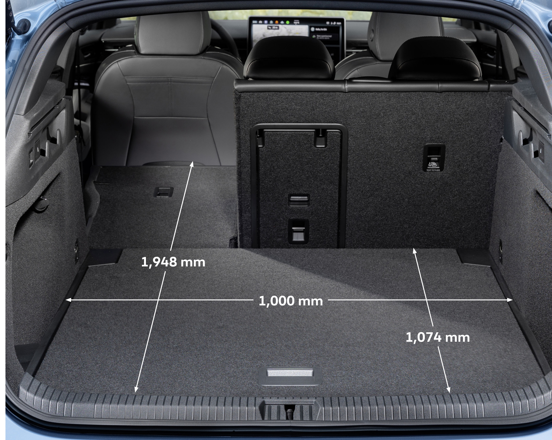
The luggage compartment dimensions of the ID.7 Tourer Pro S 2 .
