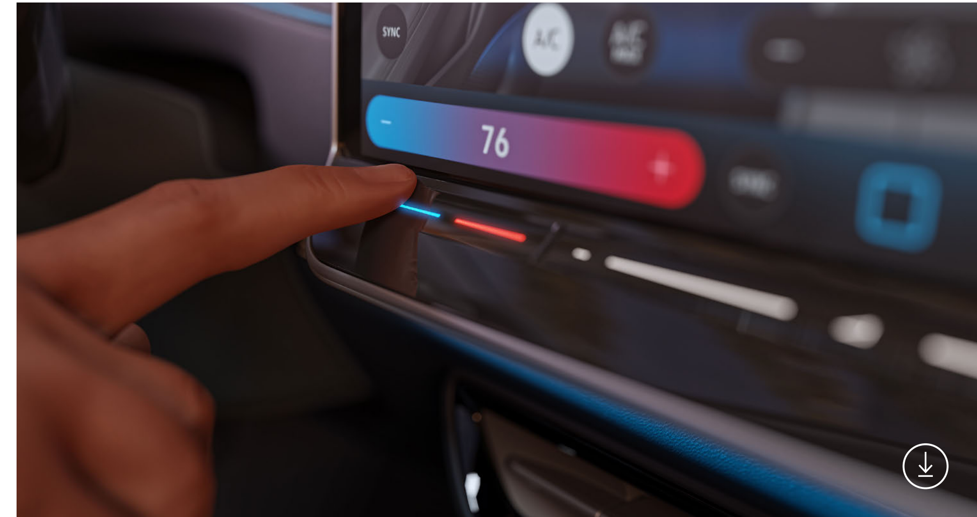
The climate control system can be operated via illuminated touch sliders.
