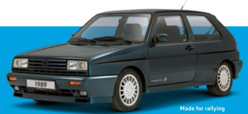
With all-wheel drive plus scroll-type supercharger and designed for motorsport: the Golf II Rallye G60 caused a stir from March 1989.
