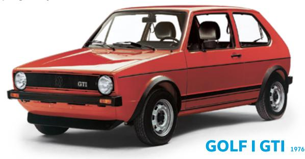
When Volkswagen presented the Golf GTI at the 1975 International Motor Show, it was astonishing to see 110 horsepower in such a discreet package. The sporty saloon with injection technology and a kerb weight of just 810 kilogrammes offered incredible performance at the time with a top speed of 182 km/h and acceleration from 0 to 100 km/h in 9.0 seconds. Production
