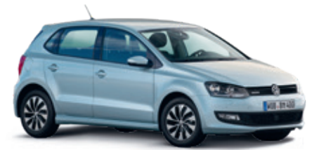
POLO V BLUEMOTION, 2009 Economical with new three-cylinder TDI with common rail injection.
