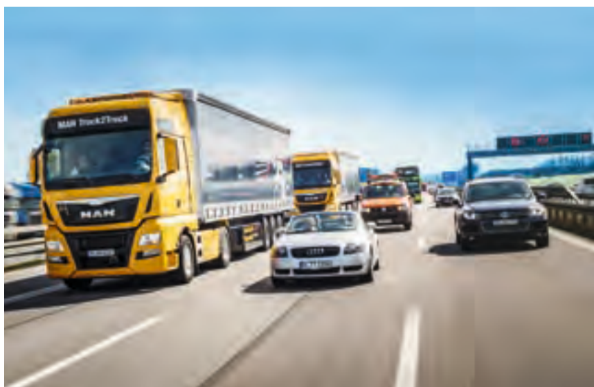
Test drive on the A9: Two digitally linked HGVs test out platooning technology. The driver in front controls both vehicles. The driver in the truck behind only intervenes in case of emergency.
