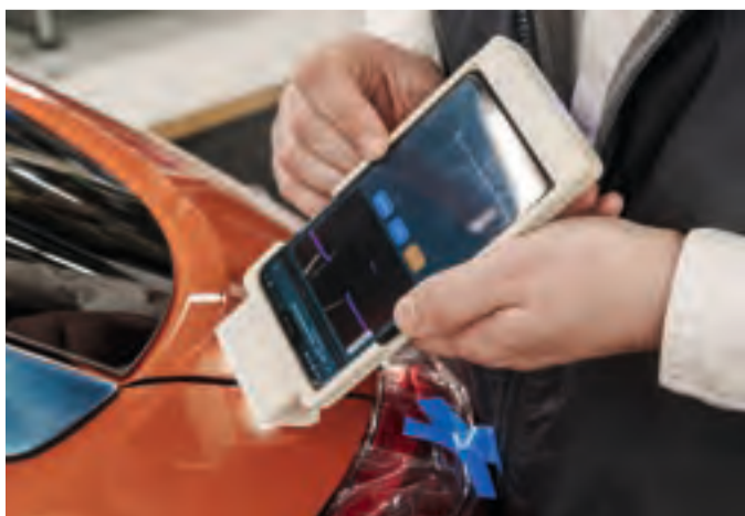
New tool: This measuring device makes it possible to take automatic and digital measurements of spacings and inclusions in all glass types.
