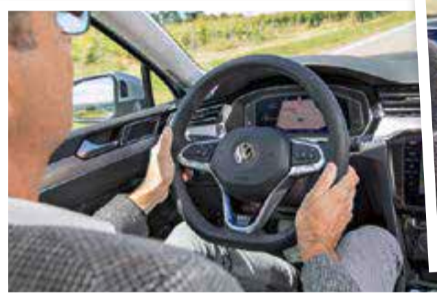
Capacitive steering wheel detects the driver's touch.
