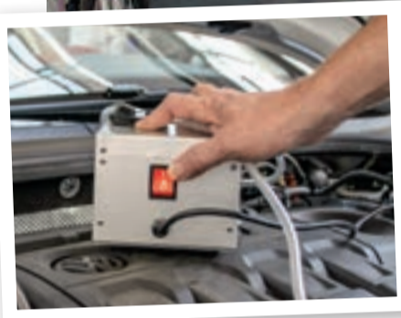
New method: Andreas Hummel (not one of the idea's submitters) works with the electric vacuum pump in the customer service workshop at the Wolfsburg plant.
