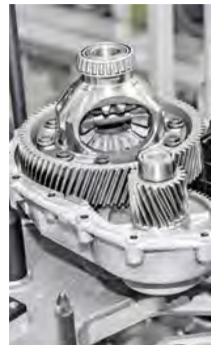
Close-up view: the single-speed gearbox and gearbox housing on the production line.
