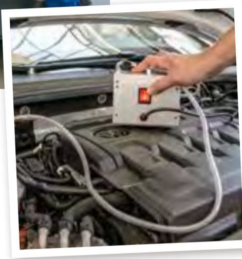
One of many good ideas: Employees proposed allowing service workshops changing coolants to choose whether they would continue to use a standard mechanical pump for venting or a new electric pump. This saves time and money.
