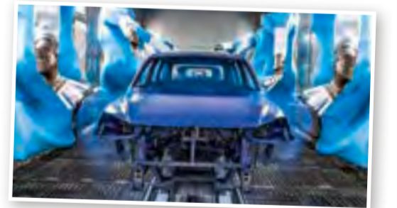
Paint shop: A load-dependent volume flow control system saves electricity and natural gas and reduces CO 2 emissions.
