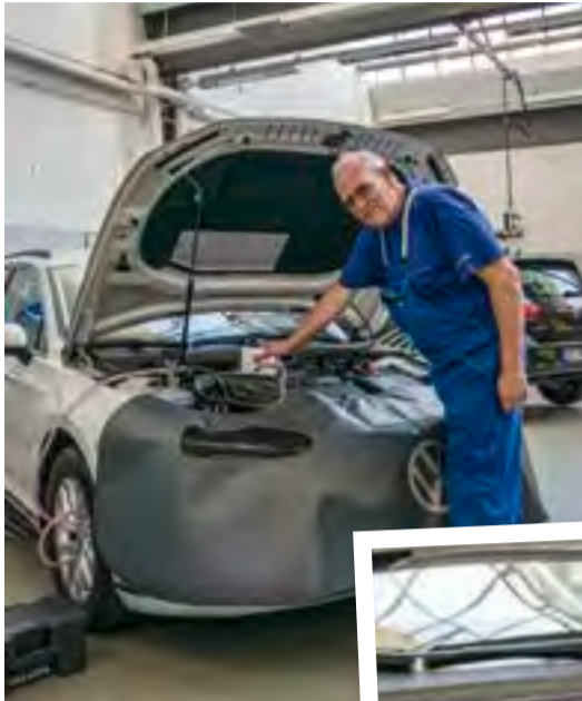
One of many good ideas: Employees proposed allowing service workshops changing coolants to choose whether they would continue to use a standard mechanical pump for venting or a new electric pump. This saves time and money.
