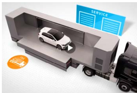
Video explains elements including the mobile exhaust gas measurement laboratory for on-site measurements of customer vehicles
