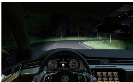
New in the Arteon: the 'Active Lighting System' that is available as an option
