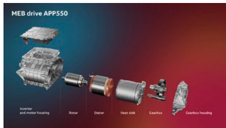
The components of the new APP550 MEB drive.
