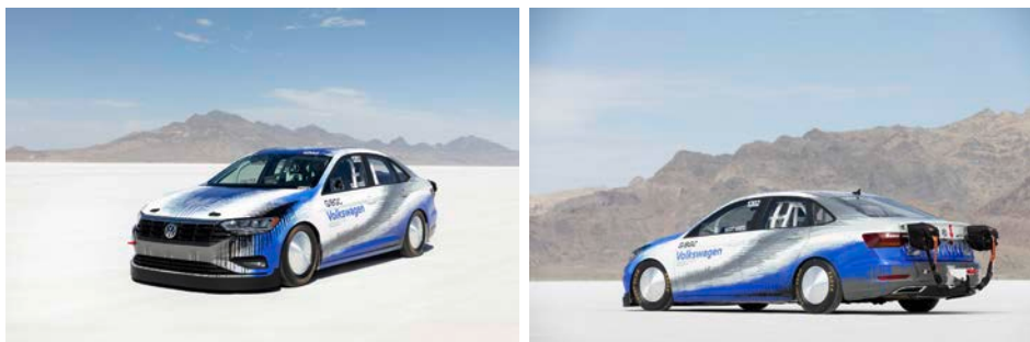
Modified Jetta sets new speed record of 338 km/h at the Salt Flats in Utah (USA) The record-breaking vehicle is equipped with two brake parachutes
